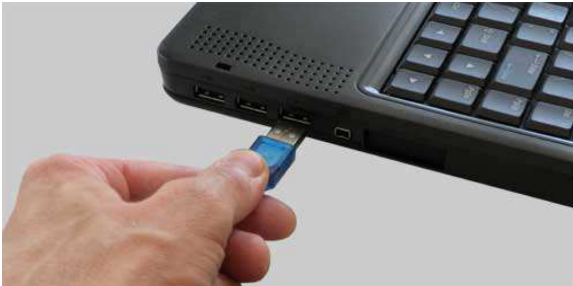
Connecting the EScan Serial Version (Using the Blue USB to Serial Bridge)
